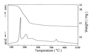
**Figure 1.** DTA-TG traces of tributylstannylated Polysiloxane 1 (21.75 mg, Run 2).
